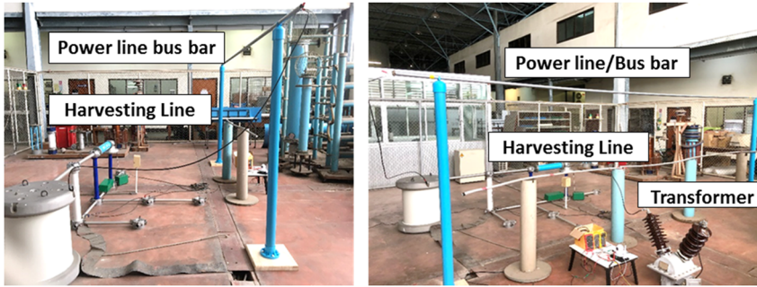
Figure 4: The actual experimental setup to validate the idea of this proposed harvester.
