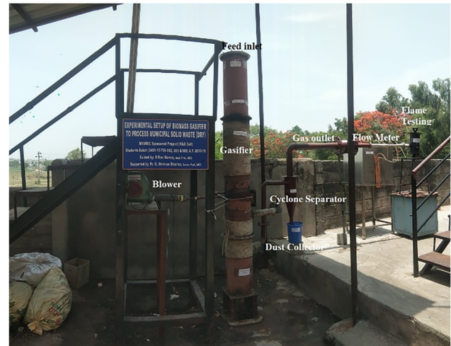
Figure 5: Photograph of the experimental setup.
