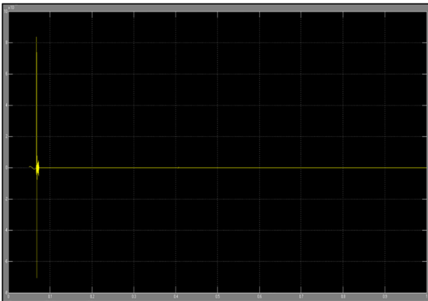
Figure 8: Self-load voltage diagram with the presence of resistor and inductor to dampen fluctuations.
