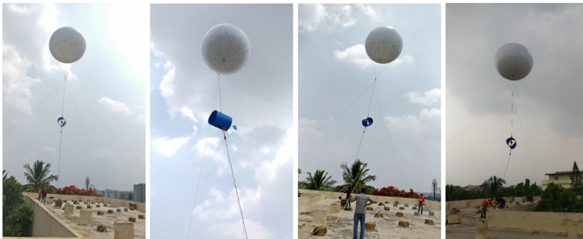
Figure 2: Airborne wind turbine experimental investigations.
