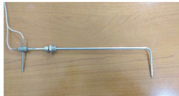
Figure 6: Pitot static tube.
