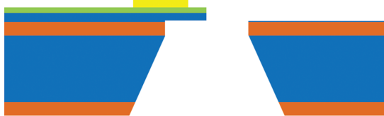
Figure 7: Steps involving bimorph fabrication using silicon on insulator (SOI) technology.
