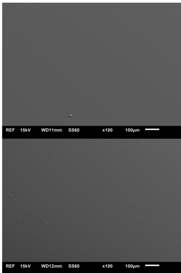
Figure 4: SEM image of spin-coated pristine (left) and KOH modified (right) PEDOT:PSS thin films.
