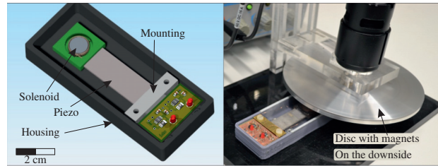
Figure 3: Concept CAD model and photography of the energy-harvesting device and testing rig.
