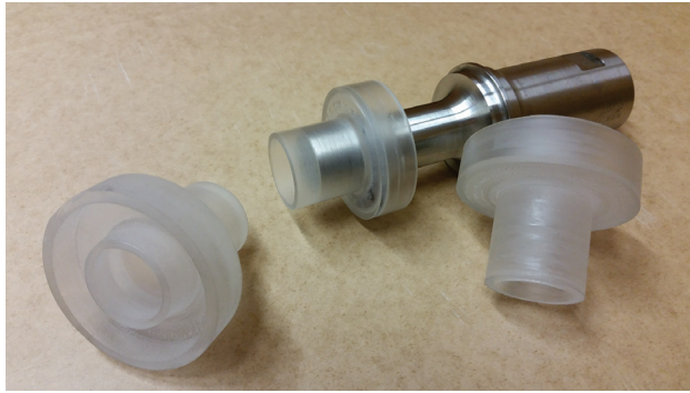
Figure 1: Plastic tools that can form a circular capillary around a transducer's tip.
