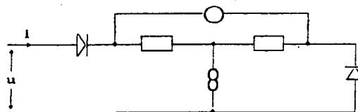
where — denotes a nullator (i. e. an element with  $u = 0$  and  $i = 0$ ) and — a norator (an element for which all points in the  $u / i$  plane describe possible states). The current / voltage diagramm of this circuit is
