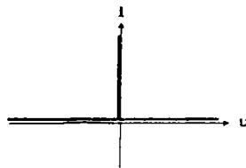
In the equations of motion [8] of such a circuit, the 1-form  $\alpha := u \cdot di$  occurs which is evidently zero. According to the formal rules of exterior differentiation, one would obtain  $d\alpha = du \wedge di$  which is different from zero at the origin. Now Smale's theory of electrical circuits shows that these forms may simply be ignored in order to get the correct equations of motion. This is the engineer's argument for passing over to the above-mentioned equivalence classes.
