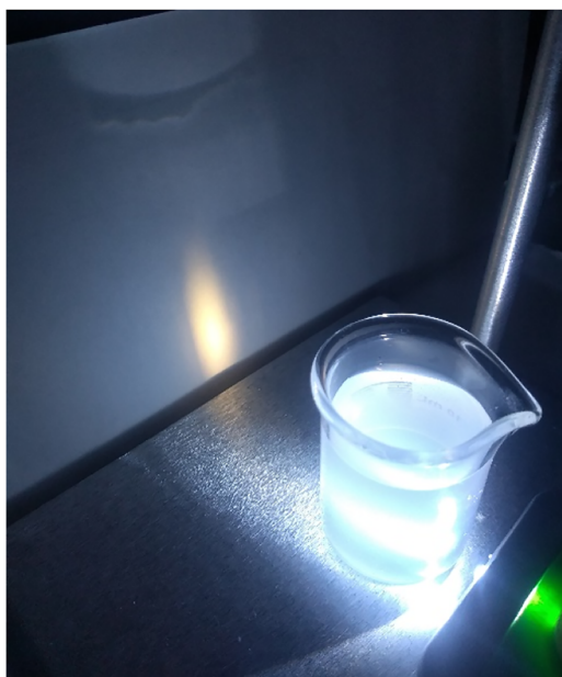
Figure 3: Rayleigh scattering in a colloidal suspension.
