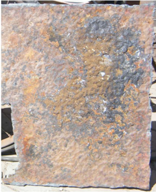
Figure 12: Corrosion on ship plate [39].
