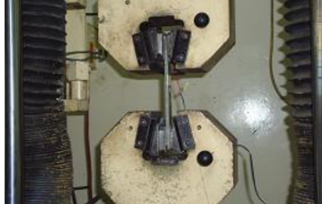
Figure 1: Tensile testing using a calibrated Universal Testing Machine.
