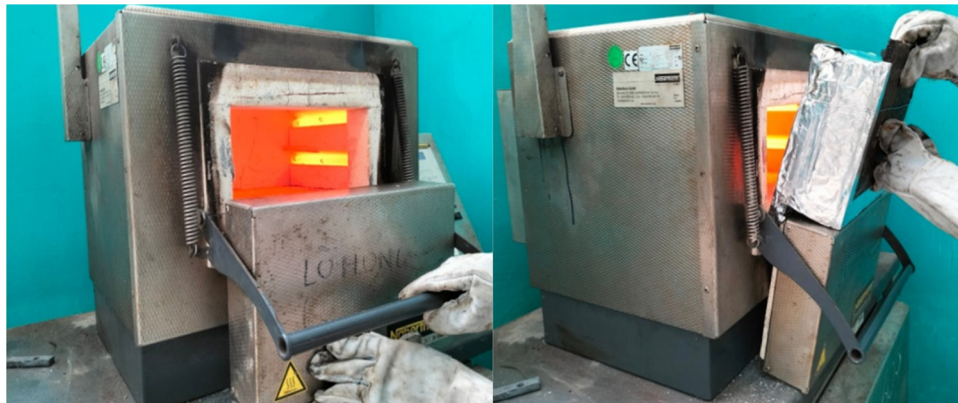
Figure 14: Setup of the specimen into the furnace.
