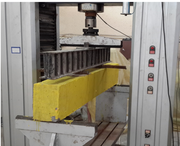
Figure 7: Test setup and loading condition for beam samples.
