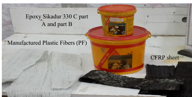
Figure 2: CFRP sheet, manufactured PFs, and epoxy.
