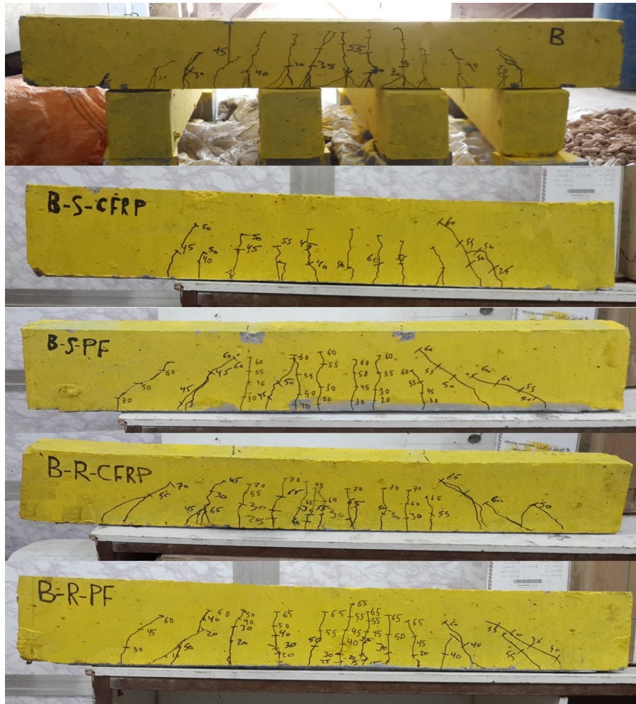
Figure 8: Cracking pattern in the tested samples.
