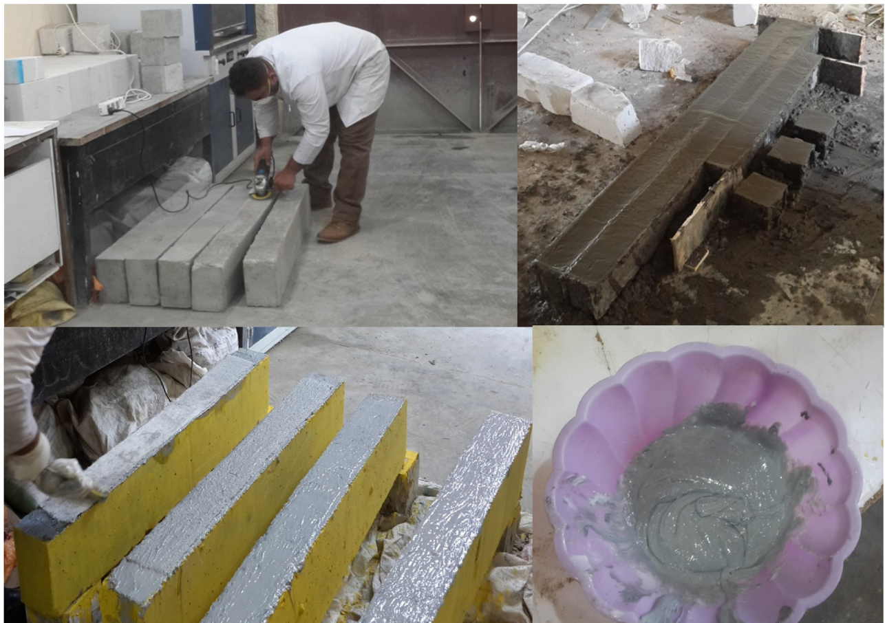
Figure 6: Casting process and strengthening of reinforced concrete beams with fibers.
