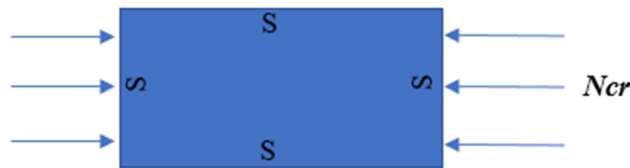
Figure 7: Schematic representation of simply supported edges with buckling load.
