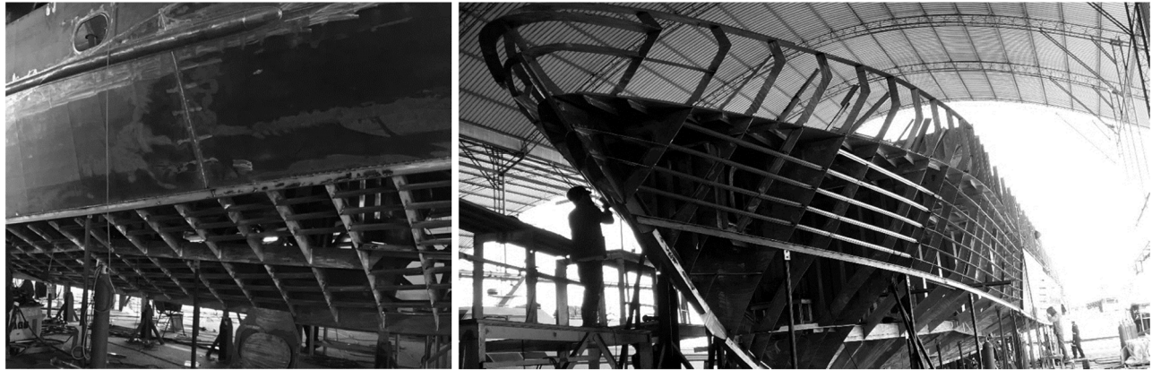
Figure 9: Structural layouts for 30 m class patrol vessels from The Maritime Affairs and Fisheries Ministry of Indonesia.
