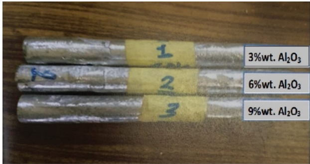
Figure 1: Nano composite samples after manufacturing
