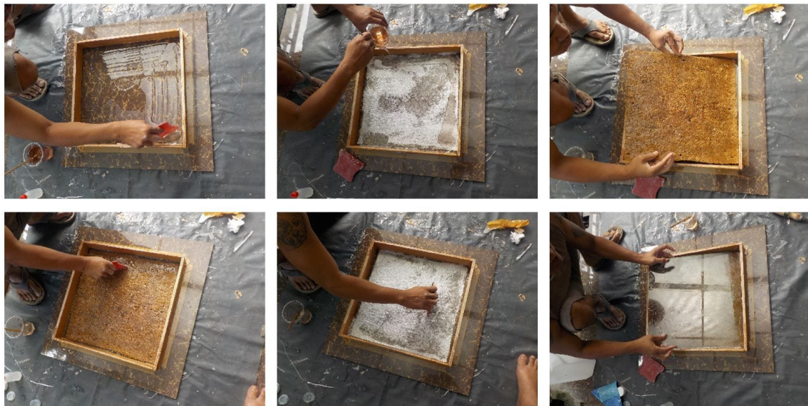
Figure 2: Lamination process using the hand lay-up method to manufacture hybrid coir and glass fiber composite material (HCGFRP)
