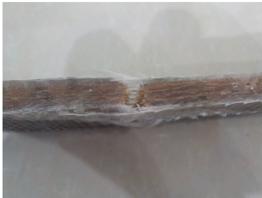
Figure 6: Fracture contour in tensile test specimen
