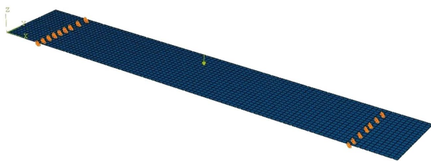
Figure 14: Bending test model for material model validation
