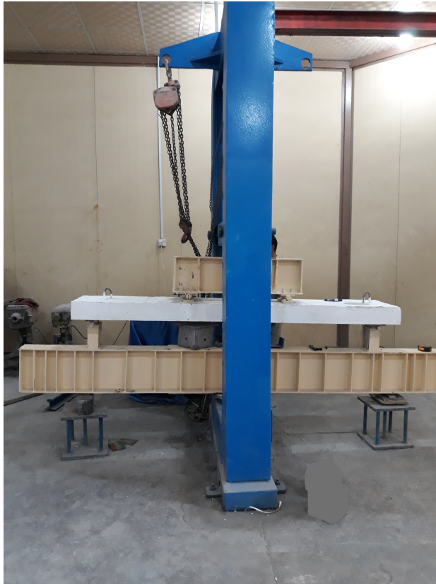
Figure 10: Flexure test machine.
