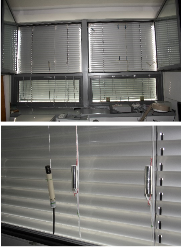
Figure 17: View of the installed sensors for measuring the physical parameters of the cavity of the double skin facade element.
