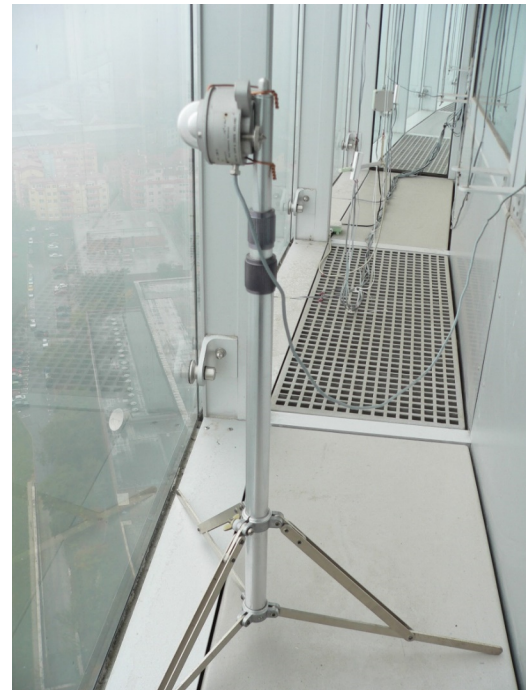
Figure 11: View into the cavity of a double skin facade with installed sensors of physical quantities.
