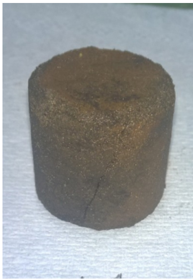
Figure 4: Unsaturated sample of the reservoir rock after testing (sample No. 1)
