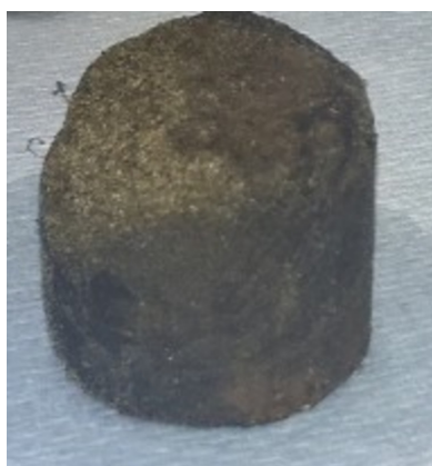
Figure 8: A sample of the reservoir rock saturated with hydrocarbon liquid after the test (sample No. 3)
