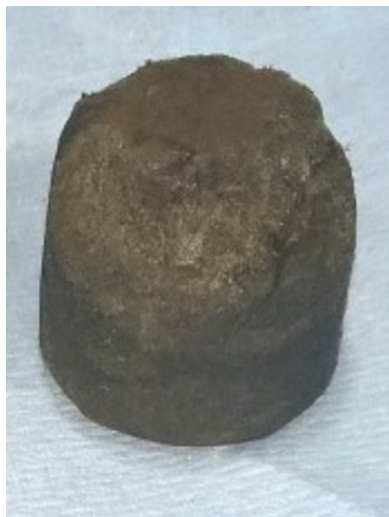
Figure 6: A sample of the reservoir rock saturated with formation water after the test (sample No. 2)
