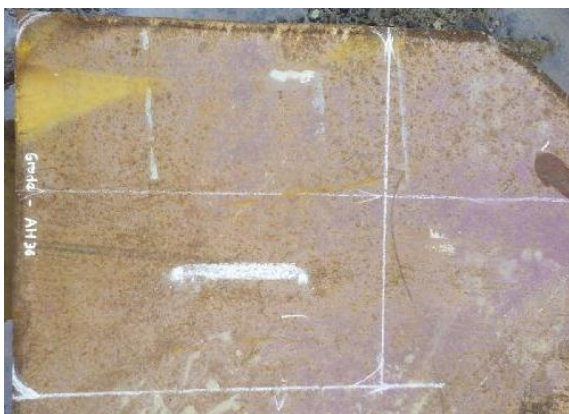
Figure 7: Repair material: steel grade AH36.
