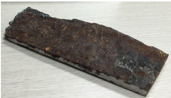
Figure 6: Destroyed material: medium-carbon steel 1030.
