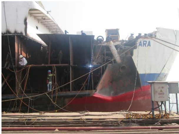
Figure 2: Repair process of side structure after a collision incident.
