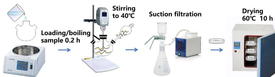
Figure 2: Schematic diagram of the recrystallization process of crude NGu.
