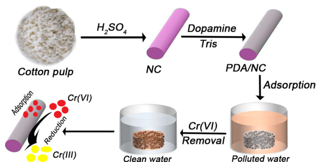
Scheme 1: Schematic illustration of the PDA/NC nanocomposite synthesis for the removal of Cr(VI) ions.
