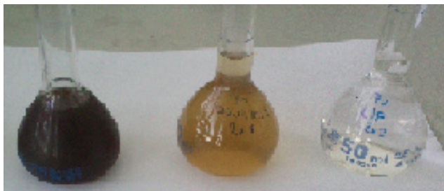
Figure 6: Compost leachate (left), after the treatment with PACl (centre) and after NF (right).
