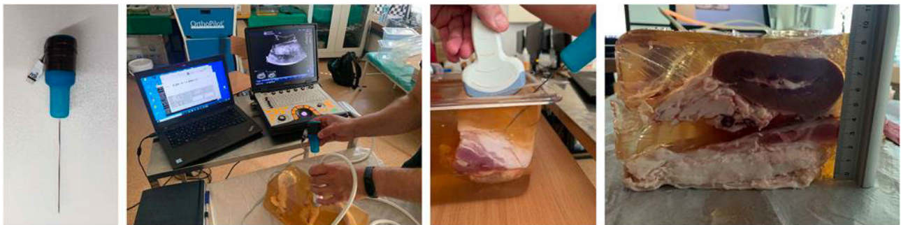
Fig. 6 Experimental setup including a synchronous US and audio data acquisition for manual needle insertions in porcine. Kidney placed in gelatine phantom — AGH, 2020.
