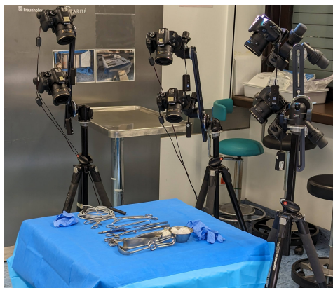
Fig. 2: Data acquisition setup. Data Acquisition at the Charite Hospital Center using six Canon 550D cameras capturing the scene on the operating stand from various perspectives.
