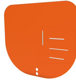
Fig. 2: CAD view of the stencil, illustrating various incision lines and two alignment holes for precise positioning on the fixture.
