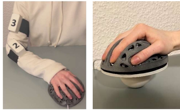
Figure 1: Input device with neutral positioning of the hand. Left: Device with the cuffs, Right: Device with tilting base.
