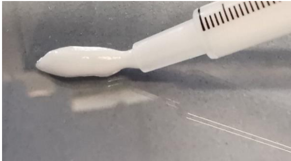
Figure 2: Two component periodontal depot consisting of TELA-NCO and CHX gel after mixing, applied by a standard 1 mL syringe.
