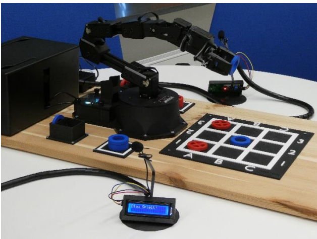
Figure 1: Hardware setup of Tic-Tac-Toe speech-controlled robotic assistant system.
