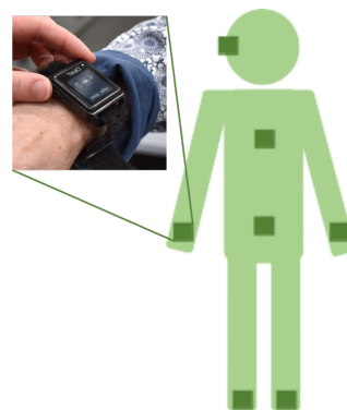
Fig. 2: APDM motion sensor and used sensor positions (ear, sternum, lumbar, right/left wrist and right/left foot).
