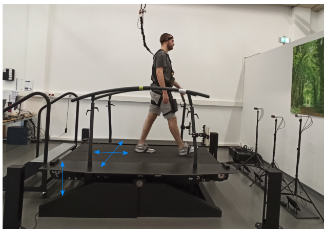
Fig. 1: Experimental setup with a MGait perturbation treadmill. The treadmill can introduce perturbations in anterior-posterior, medio-lateral and pitch direction (blue arrows)
