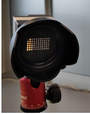
Fig. 1: The hyperspectral light-field camera used in this work. Behind each micro-lens a different spectral filter ( \lambda = 350 - 1000\text{nm} ) is located.
