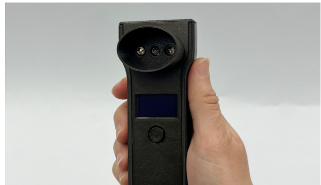
Figure 1: Hand-held prototype sensing system using infrared LEDs and a photo diode.
