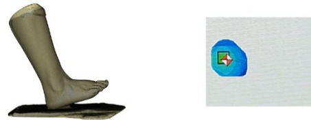
Figure 3: Geometry and load during the first contact of the foot when walking.
