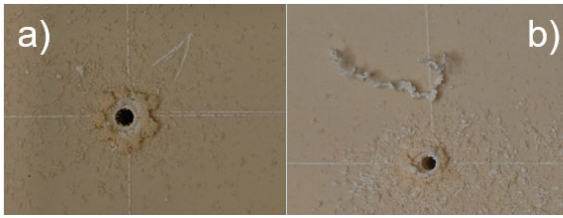
Fig. 3: Chip formation with single-lip drill a) and spiral drill b)
