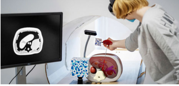
Fig. 2: Feasibility study apparatus. Phantom, world marker, needle with multi marker, RGB camera, monitor with image data, and AR glasses with 3D contents needle, path extension and anatomy.
