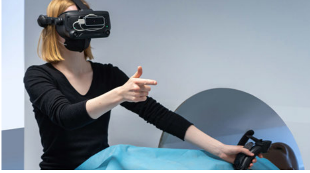
Fig. 1: User equipped with VR hardware standing next to physical mock-up of a MRI while performing hand gestures.
