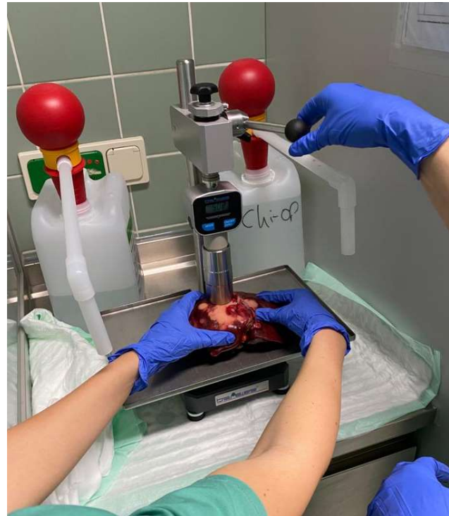
Figure 3: Ex vivo stiffness measurement of a resected liver part with tumors (brighter yellow parts) using the modified durometer.
