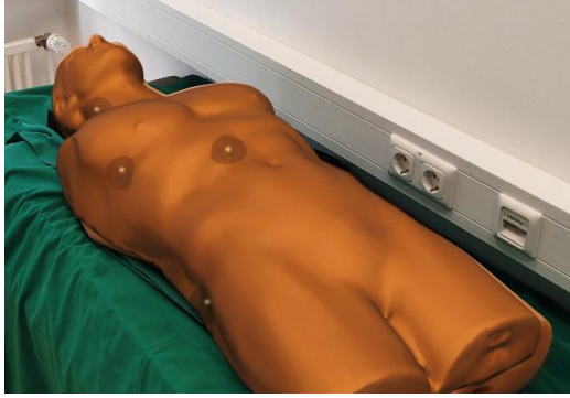
Figure 3: The HoloLens 2 user's point of view of the virtual object with the virtual markers superimposed on the real object after the PC-based registration.
