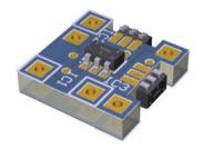
Fig. 3: Single Hall effect sensor module
