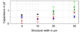
Figure 4: Coupling capacitances of parallel structures in dry environment (blue = Au, red = Pt) and wet environment (black = Au, green = Pt) with  $5 - 50 \mu m$  structural width.
