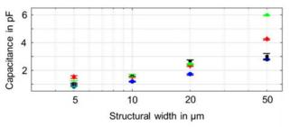
Figure 5: Coupling capacitances of overlapping structures in dry environment (blue = Au, red = Pt) and wet environment (black = Au, green = Pt) with 5 - 50 μm structural width.
