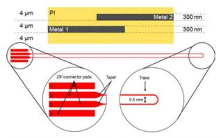
Figure 1: Structure and design of the test structures with the corresponding layer heights and important features.
