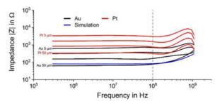
Figure 3: Measurement results of the frequency sweep with the impedances of the gold structures (black,  $5 - 50 \mu m$  structural width, dry and wet state), platinum structures (red,  $5 - 50 \mu m$  structural width, dry and wet state) and a simulated HFSS-test structure (blue,  $50 \mu m$  structural width, dry and wet state).
