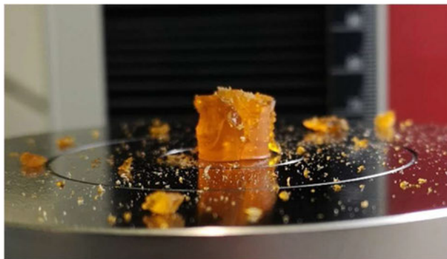
Figure 2: A burst-like fractured test cylinder of C1.
