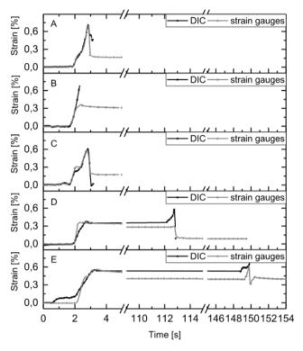
Fig. 3: Local strains determined with DIC and strain gauges.
