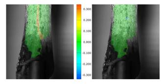
Fig. 2: Radial (left) and axial (right) strains determined with DIC on medio-lateral porcine bone surface.
