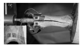
Fig. 1: Prepared porcine femora with fracutres medio-anterior determined using DIC and strain gauges.
