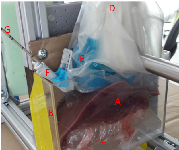
Figure 1: Holding structure with porcine liver (A), holding box (B), Aquaflux gel pads (C), linear 9L probe (D), custom 3D printed transducer holder (E), Verza needle guide bracket (F) and bipolar RF needle (G).
