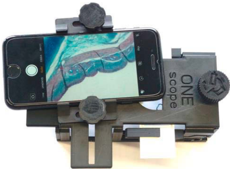
Figure 3 Assembled microscope with smartphone.
