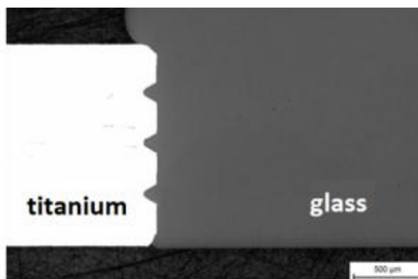
Figure 6: Titanium implant with optical window (top) and SEM image of titanium-glass-interface (bottom)
