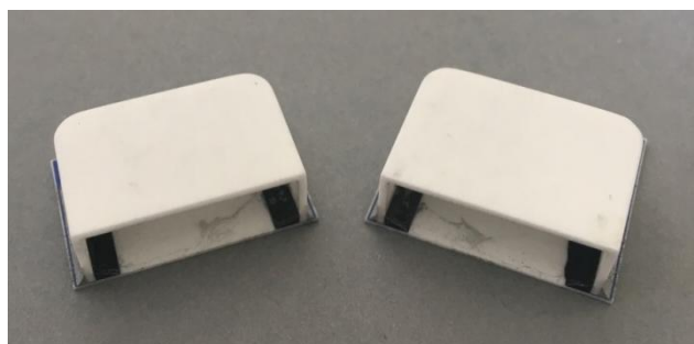
Figure 5: Cross section of a closed ceramic implant to see the internal sealing with molten epoxy
