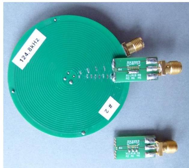
Figure 1: Extracorporeal device. Separate calibration circuit (bottom right). The rear SMA connector leads to the class-D amplifier.
