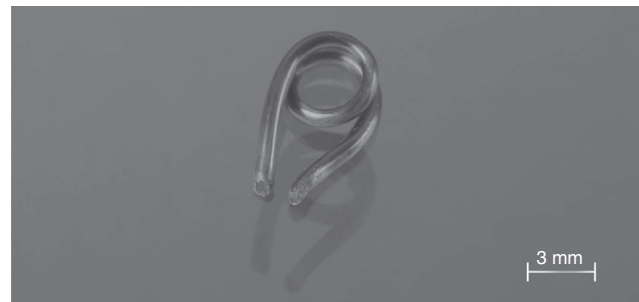
Figure 5: Helical torsion spring made from unidirectional reinforced PA12/CF.
